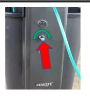
**OPERATING YOUR O₂REMOTE**: push the power switch to turn on power. Push either "IN" or "OUT" on the remote to operate. Turn speed dial to adjust speed.
